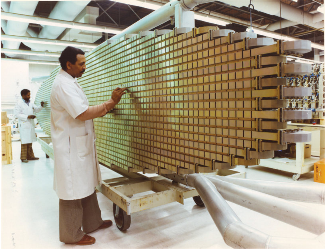
Figure 6.29 AWACS antenna array of waveguide slots. (PHOTOGRAPH COURTESY: Northrop Grumman Corporation).
